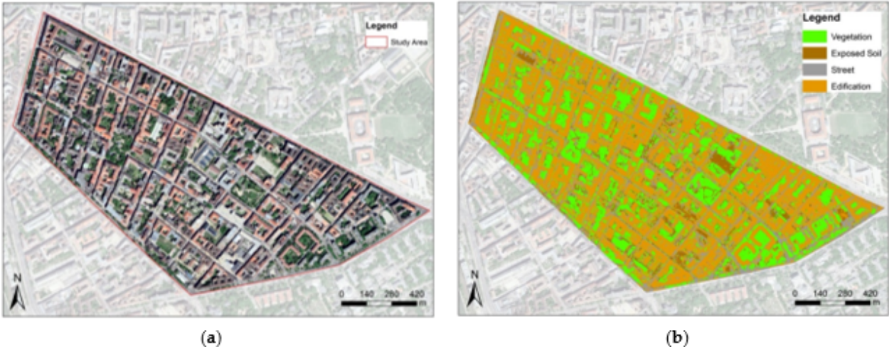
Figure 3825: Consolidation of the greenspace system. (a) Satellite image of 2021. Based on the morphological analysis, it is clear that the intervention has reached its stage of maturity; (b) implementation of green infrastructure is almost complete, and there are few areas marked as exposed soil. Source: by author.
